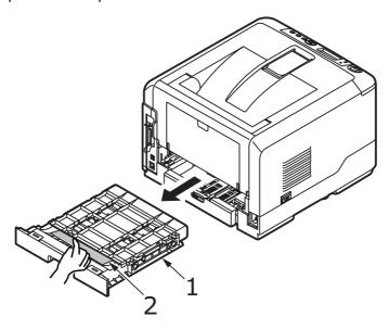
• If the paper is difficult to remove, push the duplexer cover in the direction of the arrow on the top, then raise the cover and remove the paper.
